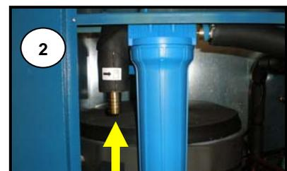
3.- Connect the outlet water pipe to the hose carrier located at the pump outlet. See the identification labels.
