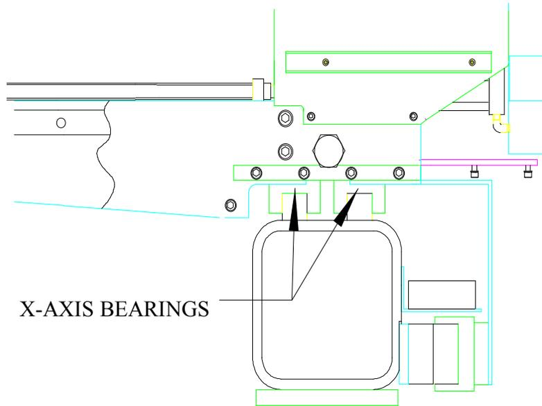
**Figure 5.5 - X-Axis Bearing Rails**
