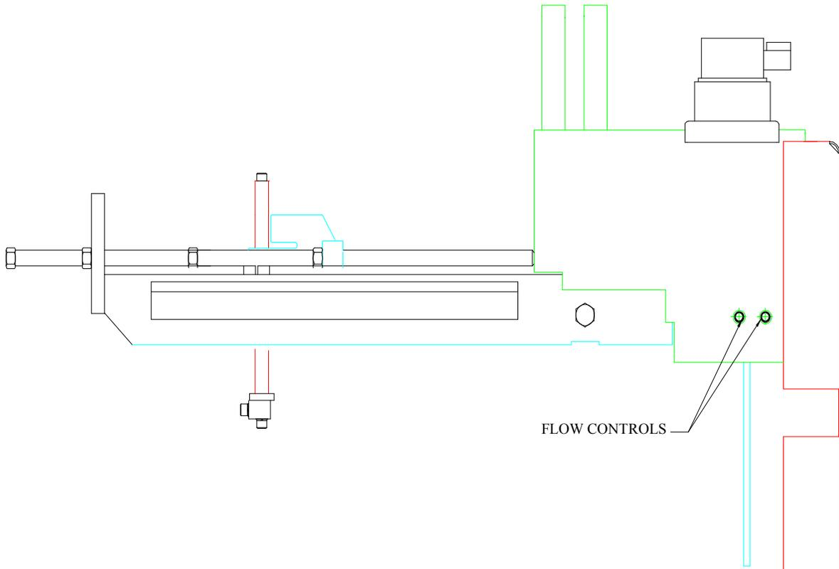
**Figure 4.2.6 - Low Speed Flow Controls**
