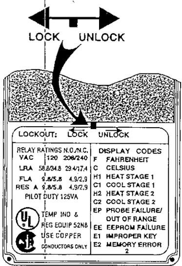
Figure 4: Lockout Switch
