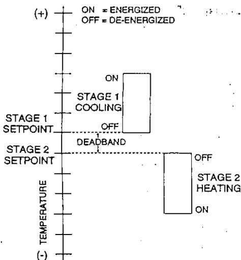
Figure 3: One Stage Cooling and One Stage Heating Example
