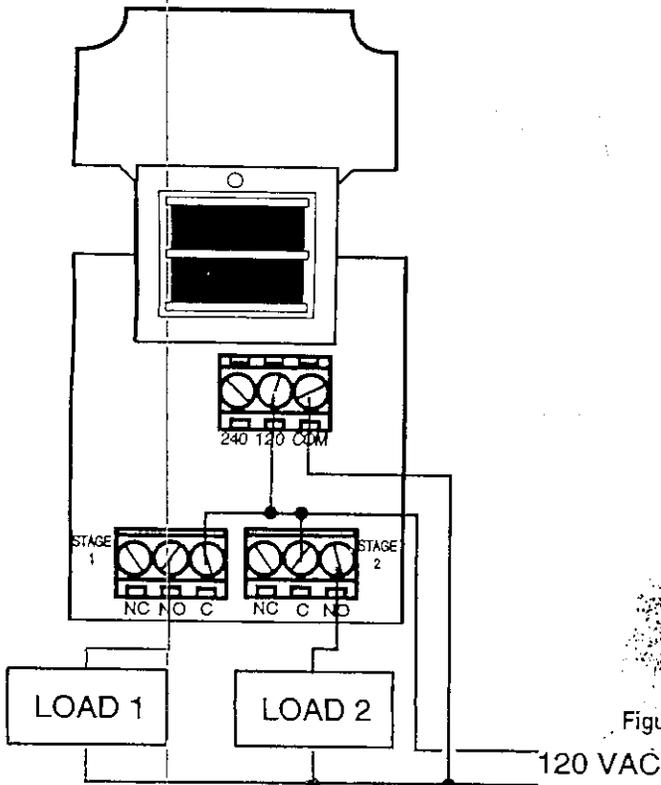
Figure 6: Typical Line Voltage Wiring Diagram.
