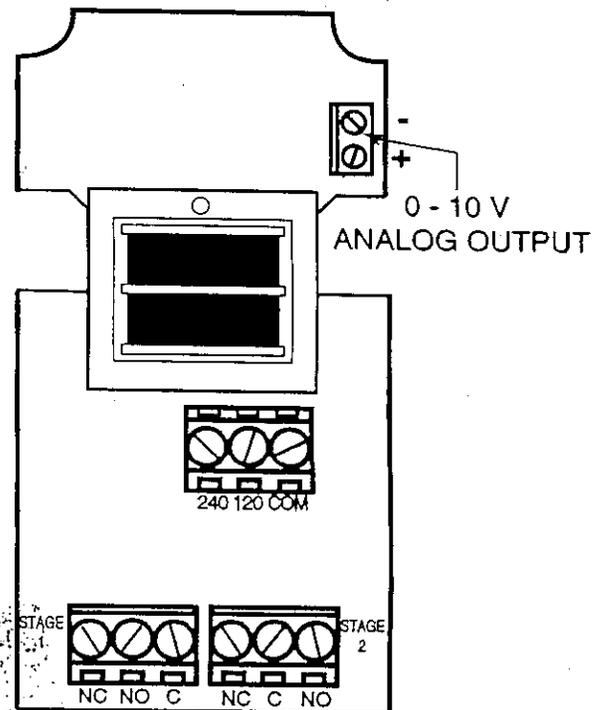
Figure 8: 0-10 V Analog Output Located on Power (Lower) Circuit Board.
